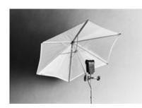
A bounce umbrella is an easily positioned source of soft light. Aim your flash unit at the umbrella, and the reflected light output is enlarged and thus softened as it is reflected (bounced) from the umbrella onto the subject. The umbrella's inner surface can be coated with white, silver or gold fabric. White produces soft light, silver produces harsher but still soft light, and gold produces warm soft light that's great for portraits.
